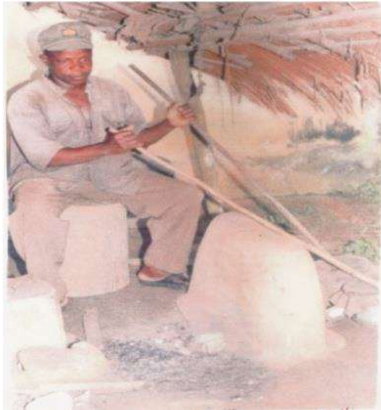
Plate 11: Isaac Wodah (Akpura) in his smithy pumping air into the charcoal fire with bellows to heat iron into reddish colour (Oct, 2005) born 1953
