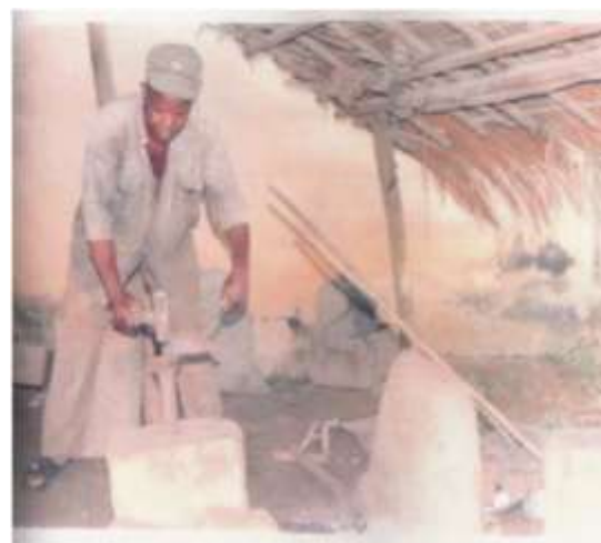
Plate 10: Isaac Wodah (Akpura) Beating and shaping a heated iron into a desired shaped of a hoe on the anvil.
