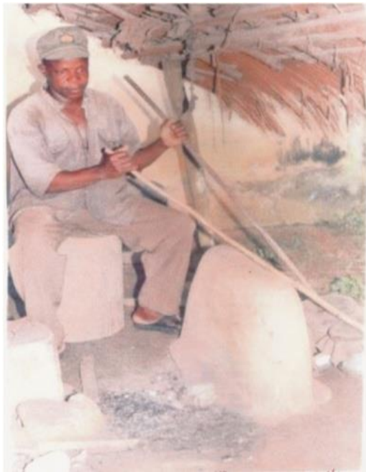
Plate 11: Isaac Wodah (Akpura) in his smithy pumping air into the charcoal fire with bellows to heat iron into reddish colour (Oct, 2005) Born 1953
